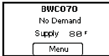
Figure 11.0a: Home Screen at Power-up (No Call for Heat)
